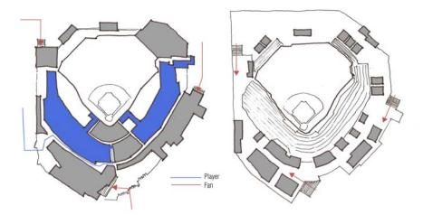
Fig 46: Plan Diagrams of Petco Park, San Diego showing separation between players and fans (Source: Author)
