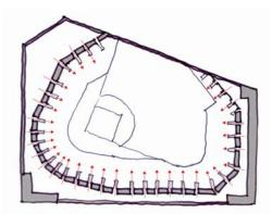
Fig 55: Plan of Fenway Park showing compressed threshold at vomitories (Source: Author)
