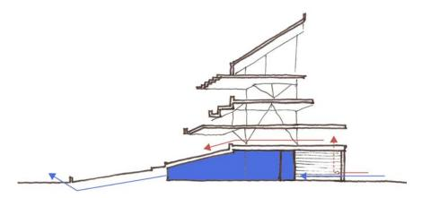
Fig 47: Section diagram of Petco Park, San Diego showing separation between players and fans (Source: Author)
