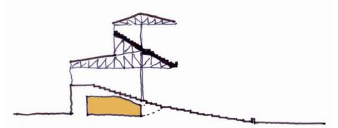
Fig 49: Section of Wrigley Field, enclosed concourse shown in orange (Source: Author)
