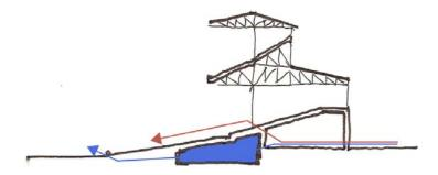
Fig 45: Section of Wrigley Field, Chicago showing concourse occupied by players and fans (Source: Author)
