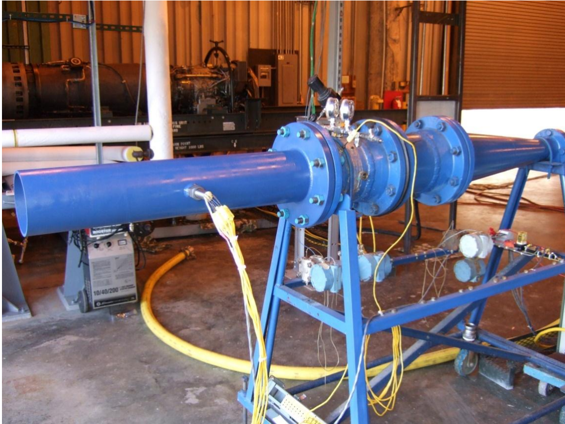
Figure 2: Photograph of the Facility Test Section Attached to the Stilling Chamber (plenum) in the UTSI Propulsion Research Facility.
