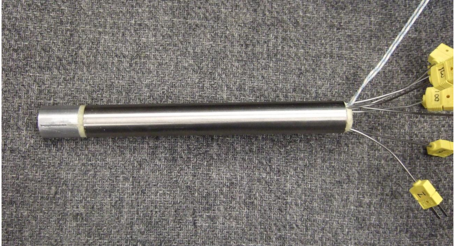
Figure 4: Photograph of the Assembled Simulated Temperature Probe.
