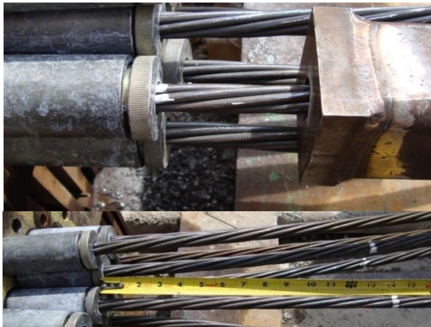
Figure 58 Initial marking and the final measurement of elongation of the strand
