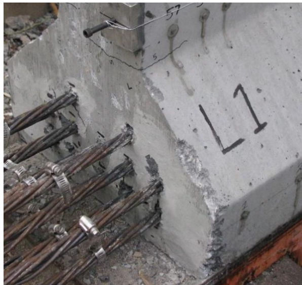
Figure 90 End L of specimen 2 designed based on Strut-and-Tie Modeling
