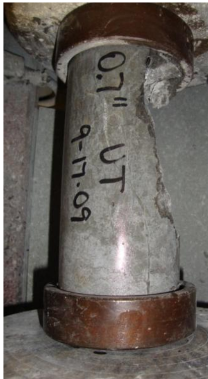
Figure 43 Concrete compression test on 4x8 inch cylinder
