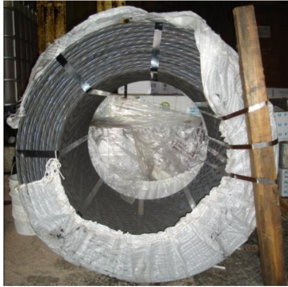
Figure 39 0.7 inch, seven wire low-relaxation strands
