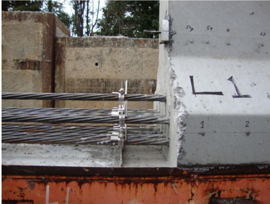
Figure 69 Strand drawn-in measurement setup
