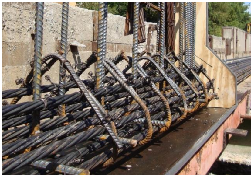
Figure 88 Reinforcement detailing for End R of specimen 2
