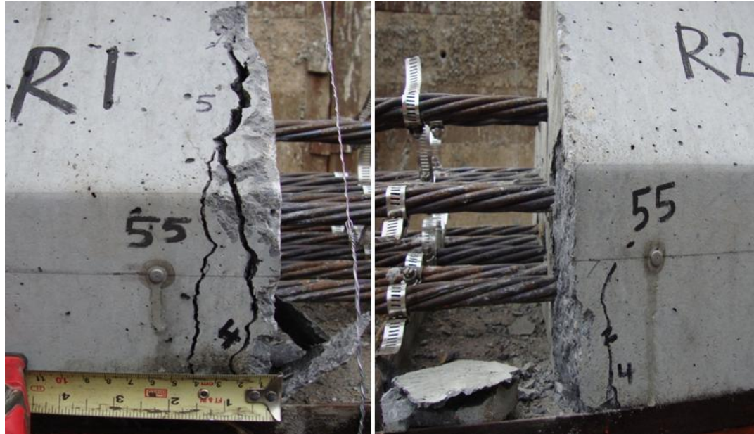
Figure 89 Both sides of End R of specimen 2 designed based on AASHTO LRFD 2008
