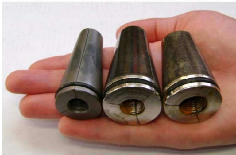
Figure 45 Jaws for 0.6", 0.62" and 0.7" diameter strands
