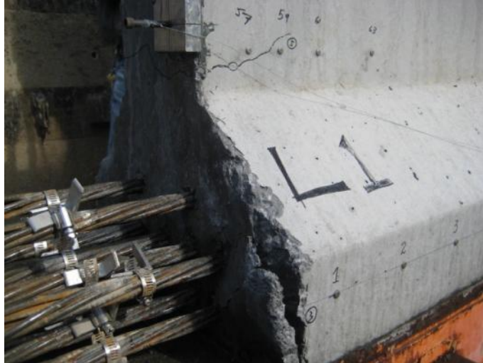
Figure 87 End L of specimen 1 designed based on Strut-and-Tie Modeling
