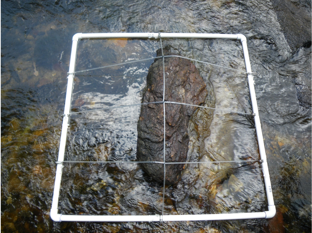
Figure 5. PVC grid used to determine substrate composition.
