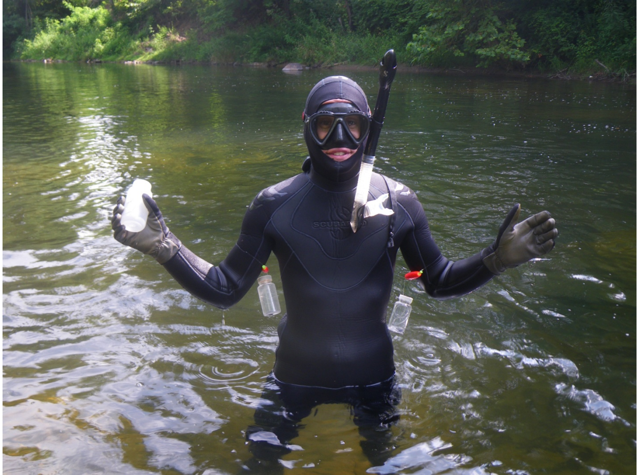
Figure 3. Snorkeler demonstrating the use of capture devices - small plastic bottles with uniquely numbered markers made of fishing bobbers, a 1.0-ounce weighted lead sinker, and 30-pound fishing line.
