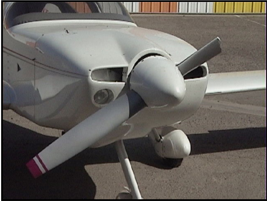
Figure 2 Author's Aircraft Following Propeller Failure (Author)
