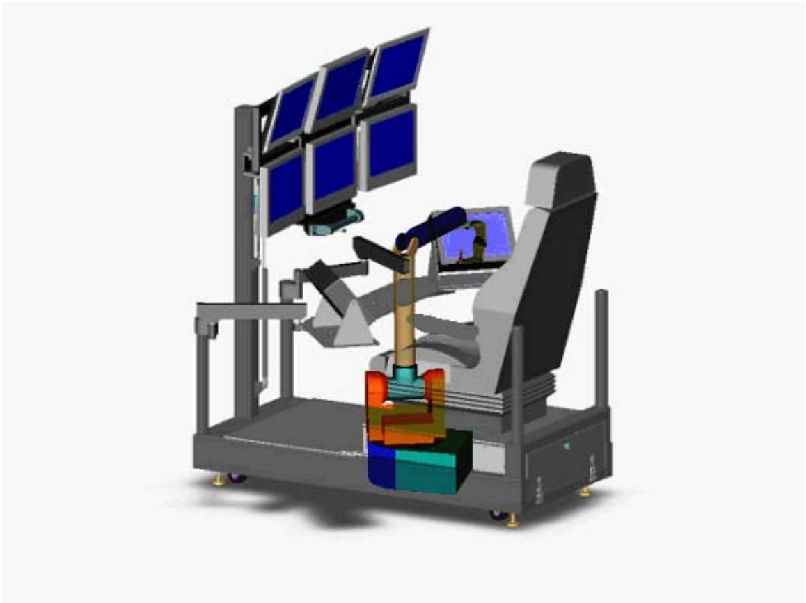
Fig 6.1 Compact Remote Console with the master manipulator WAM
