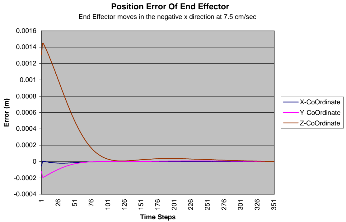
Fig 6.12 End Effector position tracking error for a different trajectory
