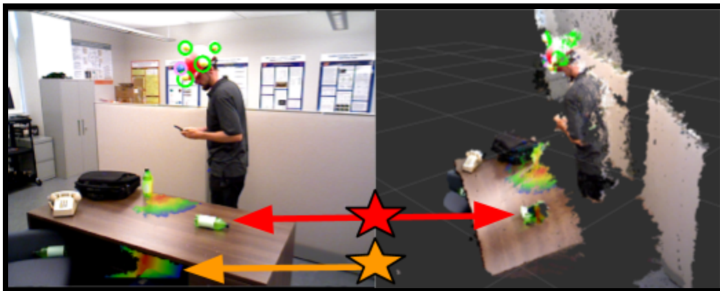
Figure 39: Point cloud scan causes object back face culling.
