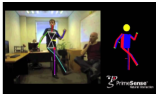
Figure 9: Skeleton extraction from natural interface sensor 5 .
