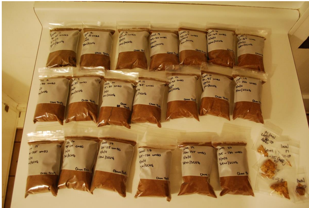
Figure H-16 Soil samples removed from Research Column HSN205E64, ready for chemical testing
