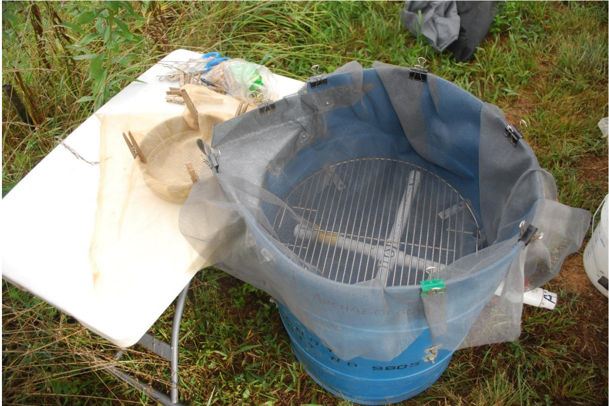
Figure 9 Modified SMAP-type flotation system used for processing the samples from both the test column and the research column
