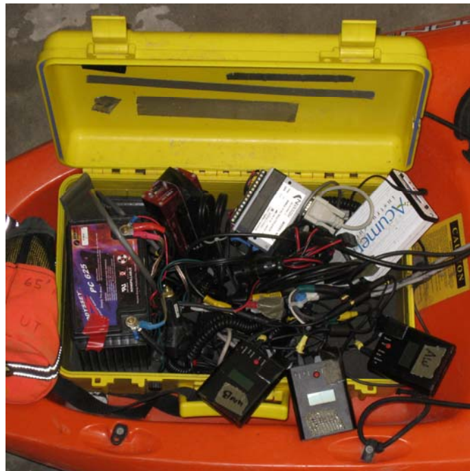
Figure 4: Battery, VMS-200, NMEA combiner, SDR, and 3 DVR recorders
