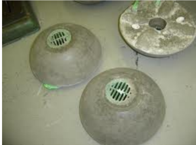
FIGURE 3 – 2. Photo of mussel silos deployed for this study. The silos are composed of a 10-kg concrete dome and a PVC inner chamber with standard 1.6-mm mesh size fiberglass screen to house the mussels. The silos were designed so that as water flows over the silo, it creates a Bernoulli effect, which draws water up through the mussel enclosure providing a continuous supply of fresh water and nutrients, while keeping mussels enclosed and easily retrieved for data collection.
