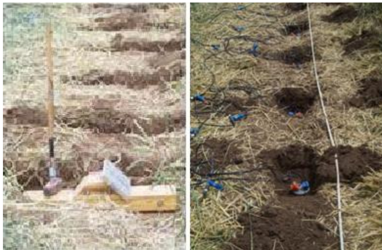
Figure 4.5. Left: Hammer and 45° wooden block source, Right: Geophone coupling location
