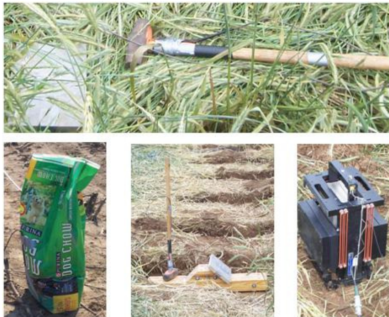
Figure 3.6. Seismic sources. Top: sledge hammer and aluminum plate. Bottom left: 22.5 kg bag of sand. Bottom center: sledge hammer and 45° wooden block. Bottom right: ELECTRO-SEIS ® vibrator.
