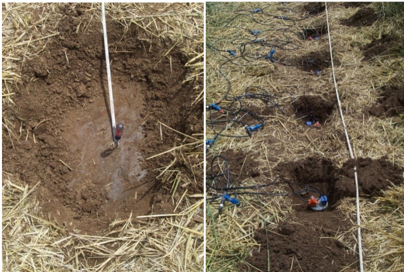
Figure 2.12. Left – Source coupling, Right – Receiver coupling.
