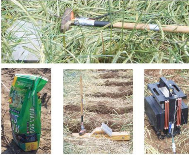
Figure 2.15. Top: Hammer and Plate source, Bottom left: 22.5kg Sand bag source, Bottom Center: Hammer and 45° wooden block, Bottom Right: ELECTRO-SEIS® Vibrator.
