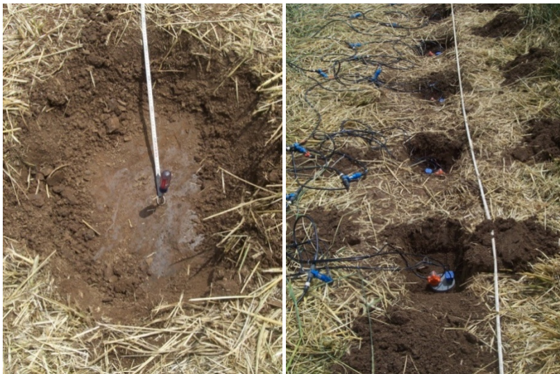
Figure 3.4. Sources and receivers. Shallow holes were used to improve coupling.
