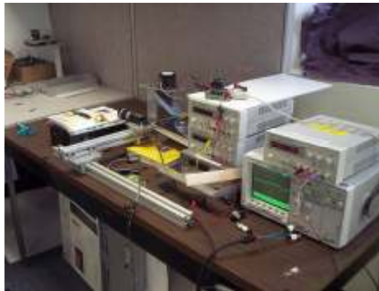
Figure 6.8: The 1 mW laser is pointed directly into the LPSM to ensure a focused point.
