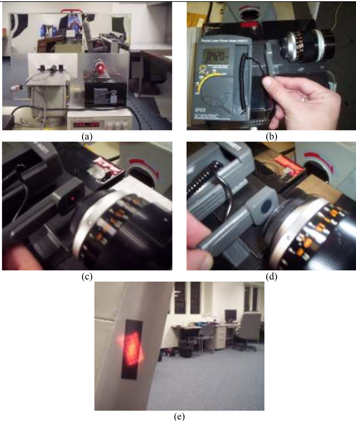
Figure 5.19: (a) The laser can be directed so that the reflection hits the lens. (b) The power of the light getting through the lens can be measured. (c) When laser light is reflected into the lens, then the light can be seen. (d) If the laser light is reflected elsewhere, then no laser light can be seen. (e) The laser is targeted so that the reflection hits the tape instead of the lens.
