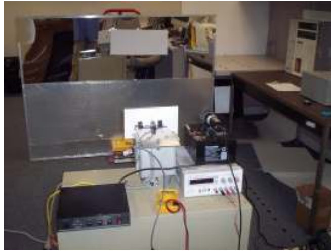
Figure 5.22: White paper was taped to the mirror to indicate the two points where the laser should be directed.
