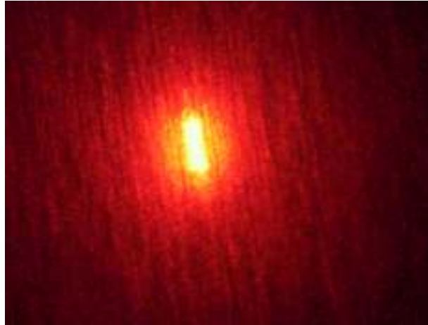
Figure 5.6: The filter caused the laser beam light to scatter, although there was a more intense spot in the middle.
