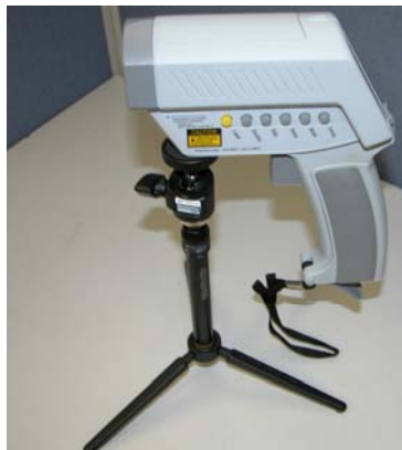
Figure 4-10: Raytek Mx4+ infrared thermometer used for temperature measurement.
