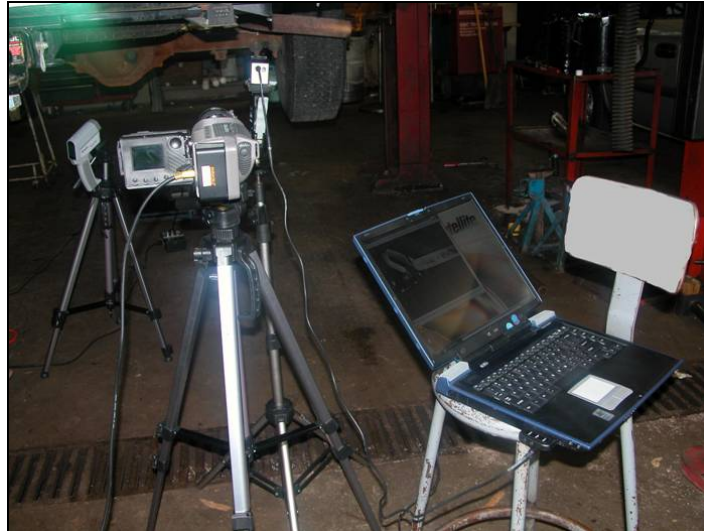
Figure 4-3: Hardware setup for thermal data acquisition. The setup includes the two uncooled infrared cameras, infrared thermometer and the laptop for controlling the devices.
