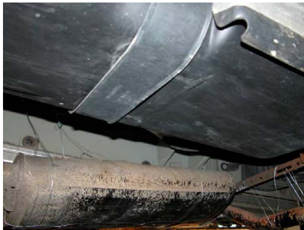
Figure 4-20: Visual image showing the false muffler.
