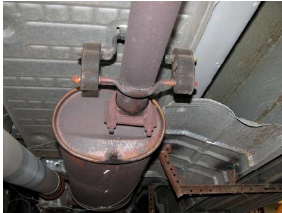
Figure 4-18: Visual image showing the real muffler connected to the exhaust system.
