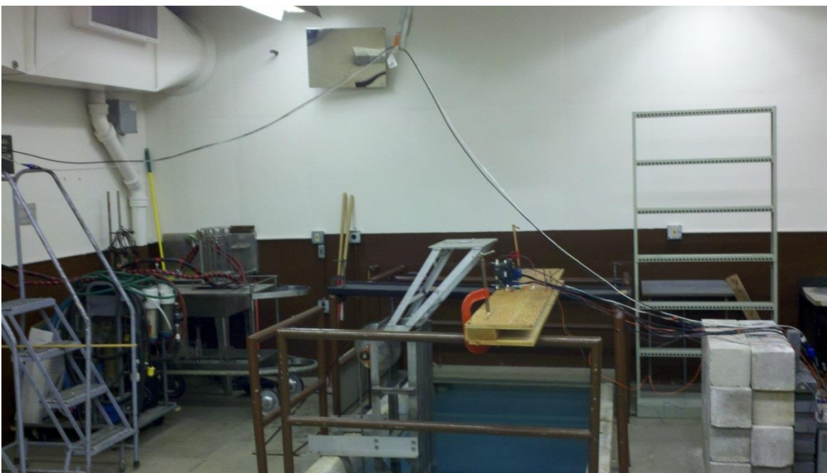
Figure 23 – Auburn's Co-60 test room where the ALD1106 and ALD1107 chips were irradiated.
