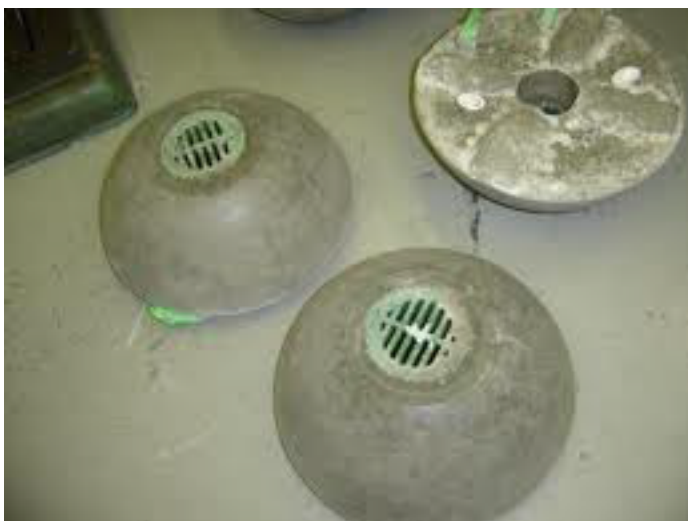
Figure 3-3. Silo. Silo width is 27 cm, height 12 cm, metal opening at top is 8.6 cm in diameter. The interior containing the mussels is 4 cm in diameter and 4 cm in height.
