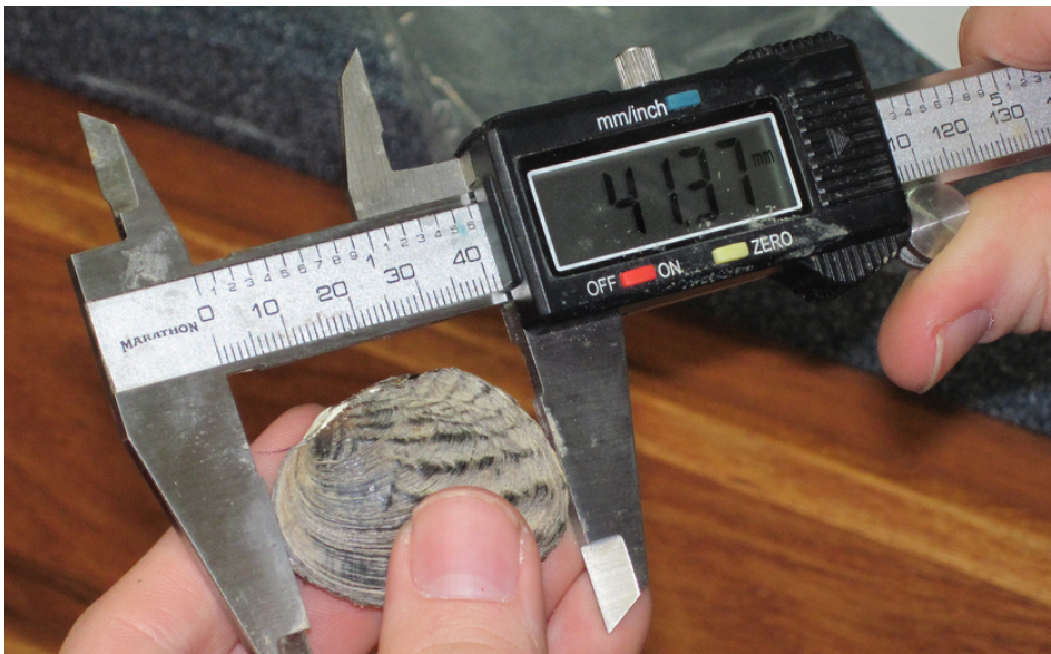
Figure 3-1. Mussel length measurement. Length measurement taken at the longest dimension (Pictured mussel is not L. fasciola or M. conradicus )
