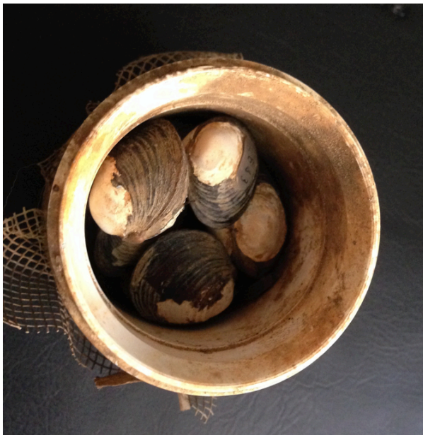
Figure 3-4. Cage. Dimensions of the cage are 9 cm in height and 6.6 cm diameter.
