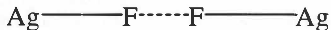
Figure 3.13: Example of a split site model for the equatorial fluorines. Each fluorine has an occupancy of \frac{1}{2} .
