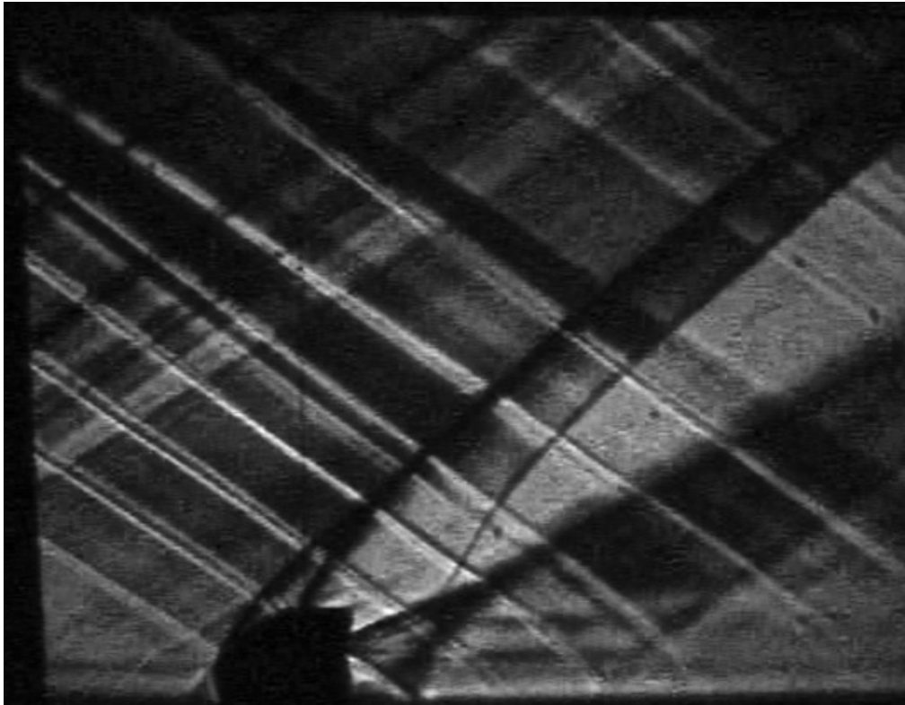
Figure 96. Test Configuration 4b: Airfoil 0° with Cavity – Schlieren Photograph
