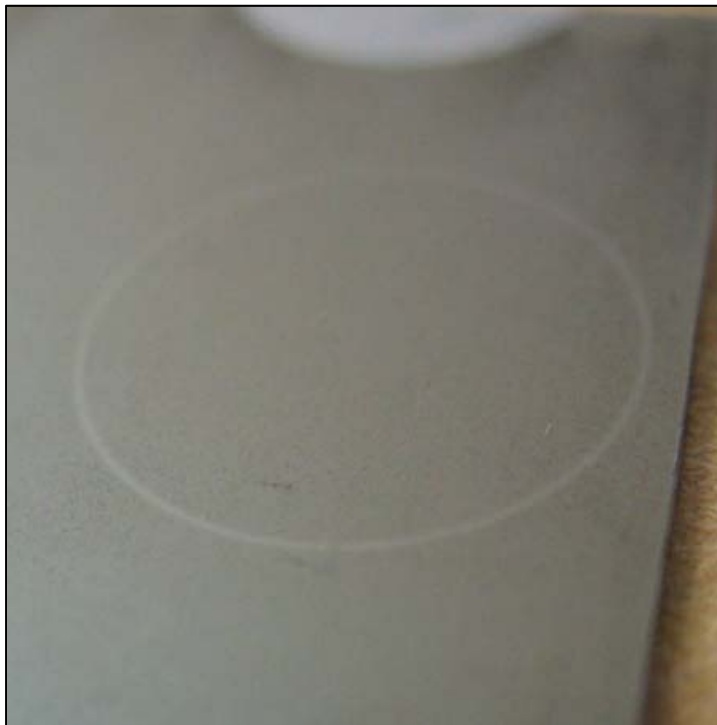
Figure 45 DLC Sample after Wear Testing with Oil Lubrication
