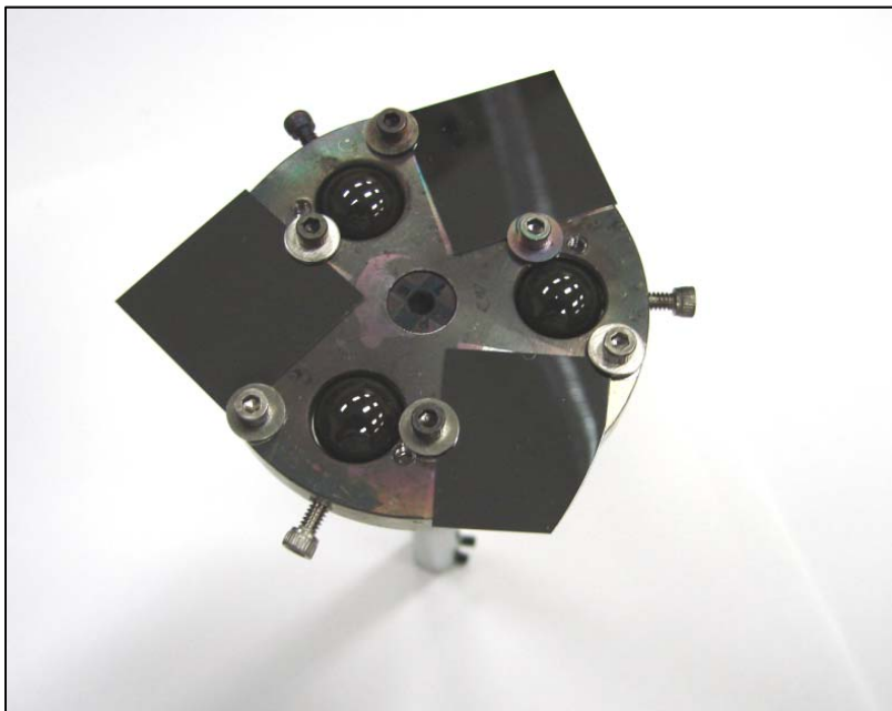
Figure 6 Silicon Wafers and Silicon Nitride Spheres Mounted on the Substrate Holder
