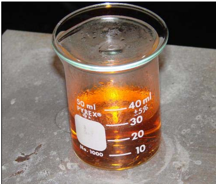
Figure 16 Samples PLD #54-2 and PLD #54-3 Soaking in a Sulfanilic Acid and Sodium Nitrite Solution
