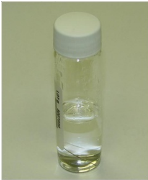
Figure 17 DLC Sample Soaking in Simulated Body Fluid
