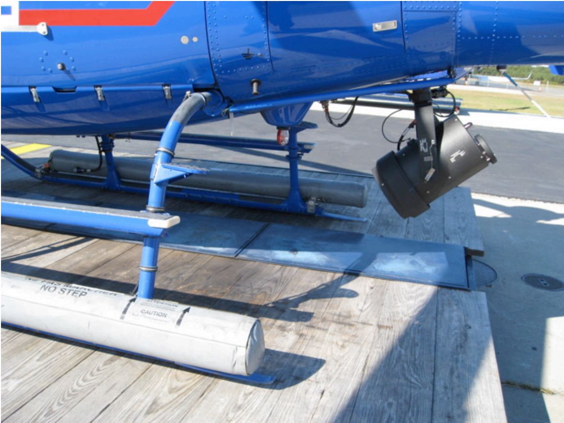
Figure 7: Example of poor systems integration. Searchlight has been restricted in allowable azimuth and elevation due to the possibility of its intense heat burning the emergency floats. This renders the light virtually useless for any practical application, especially during landing.
