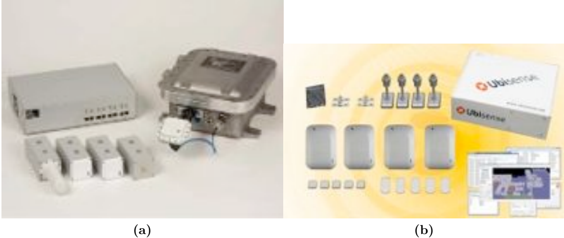
Figure 2.3: Two commercial UWB localization systems: (a) Sapphire Dart by Zebra Technologies and (b) RTLS by Ubisense. [1, 2]
