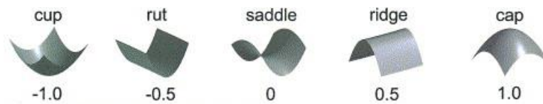
Figure 2-2: Local shape variations based on shape index, Eq. 2-15, [20]
