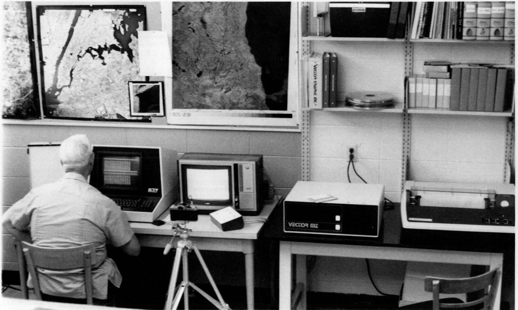
Figure 15. Carroll College, Remote Sensing Laboratory, Department of Geography, Waukesha, Wisconsin. (From Left to Right) ACT-V Video Terminal, Sony Trinitron Cathode Ray Tube (CRT), Vector MZ Microprocessor, and a Texas Instruments Omni 800/810 R.O. Terminal.
