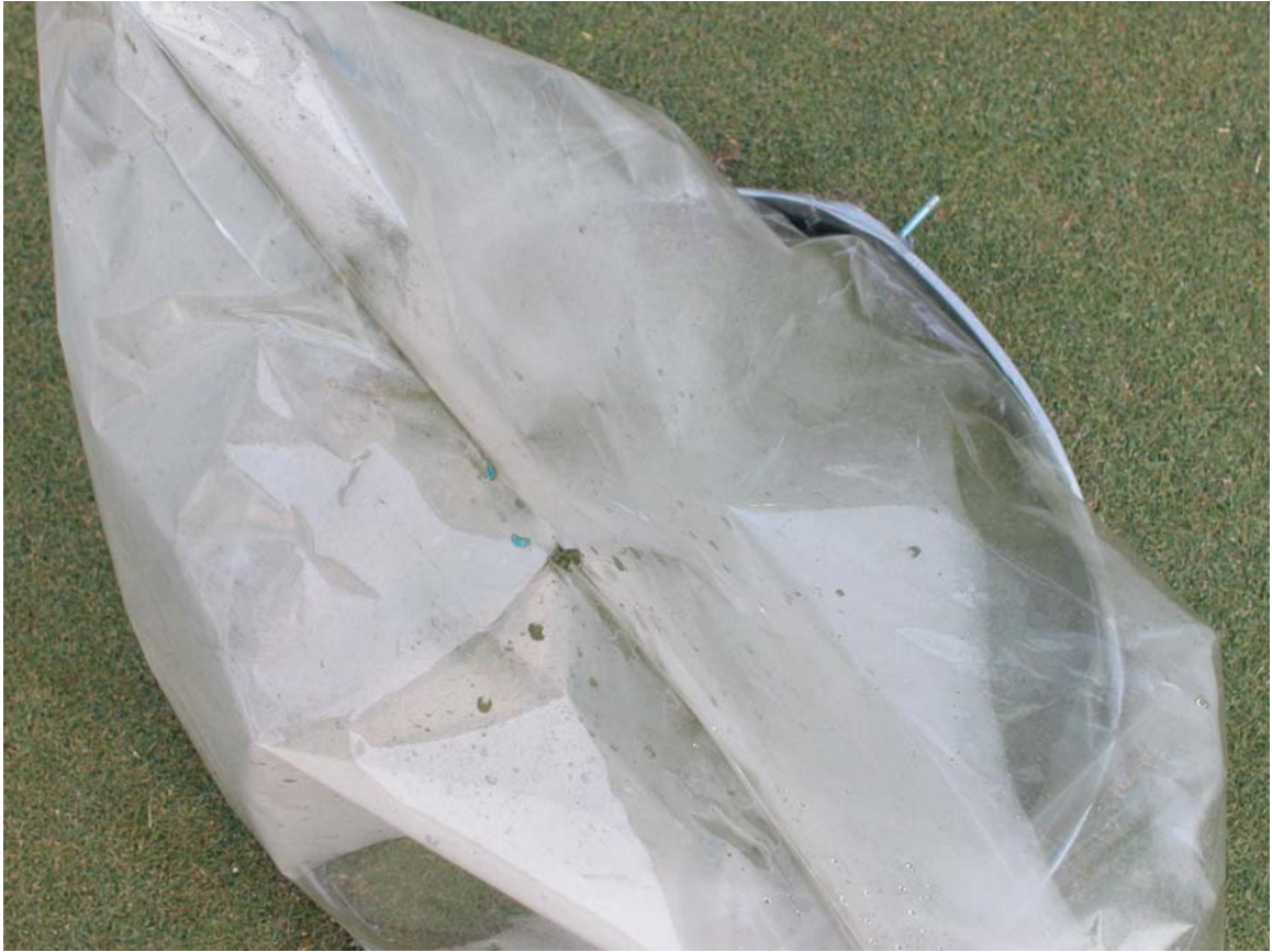
Figure A-12: Condensation observed within chambers deemed to be from too little air flow at Knoxville, TN; 17 July- 20 August, 2006.
