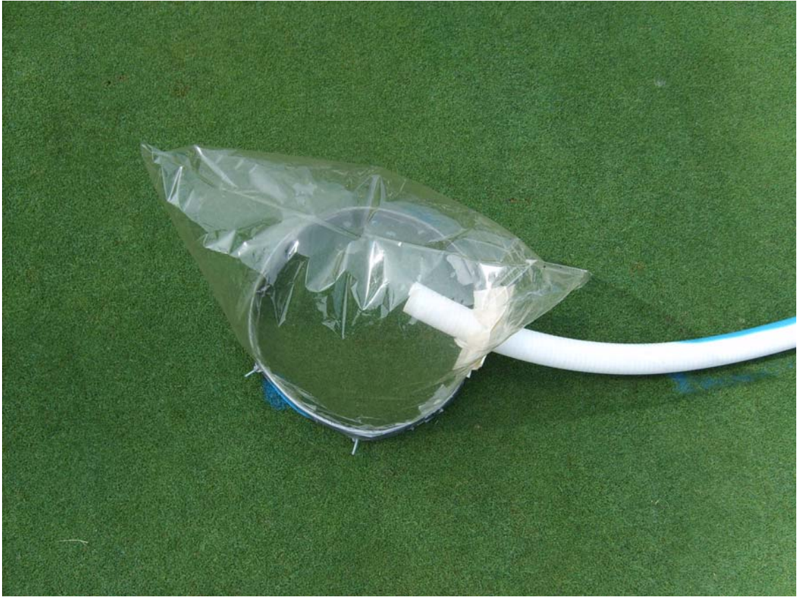
Figure A-13: No condensation observed within 2007 chambers due to adequate air flow at Knoxville, TN. 25 June- 20 August, 2007.
