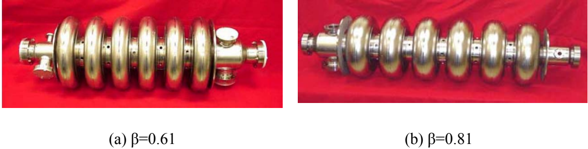
Figure 2.7: Image of the SNS superconducting RF cavities [10].
