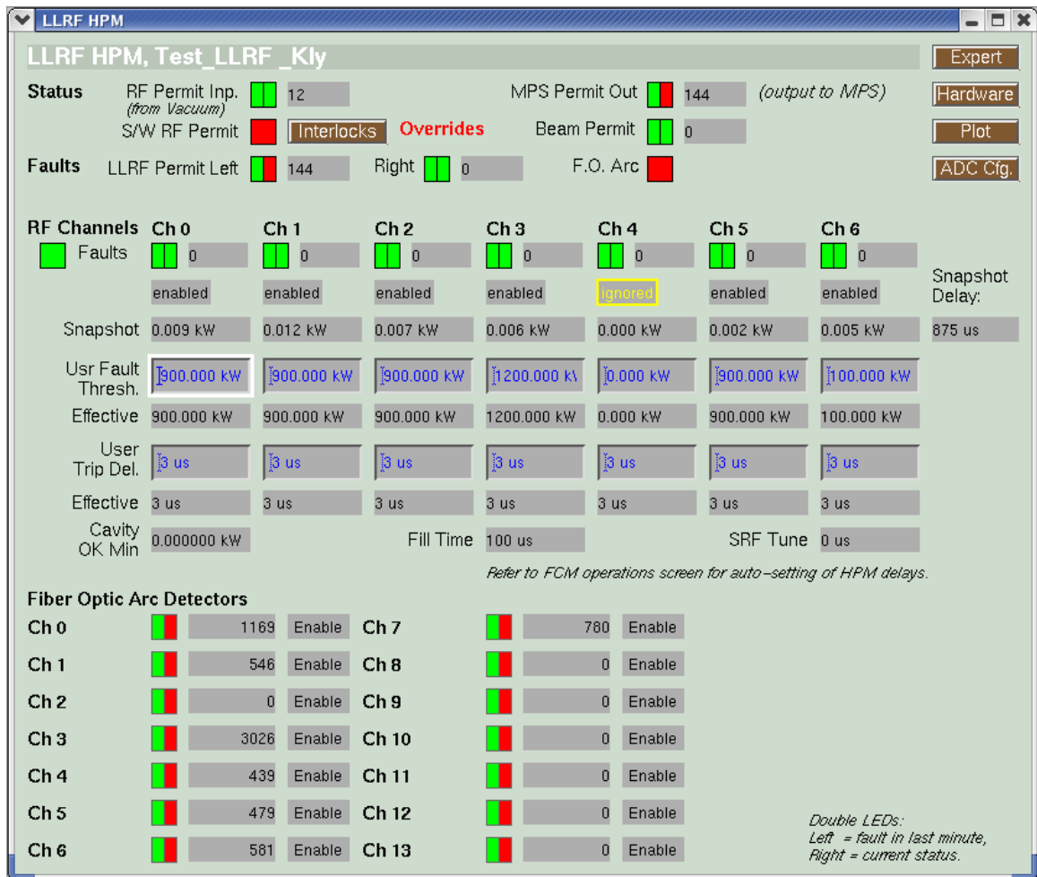
Figure 5.11: OPI screen for setting up and monitoring the instruments connected with the HPM in RF power IOC.
