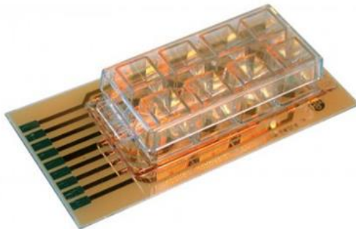
Figure 2. Commercially available gold film coplanar platform
