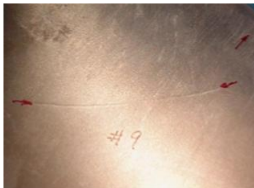
Figure 2: Example of cracking under HCF conditions [3]
