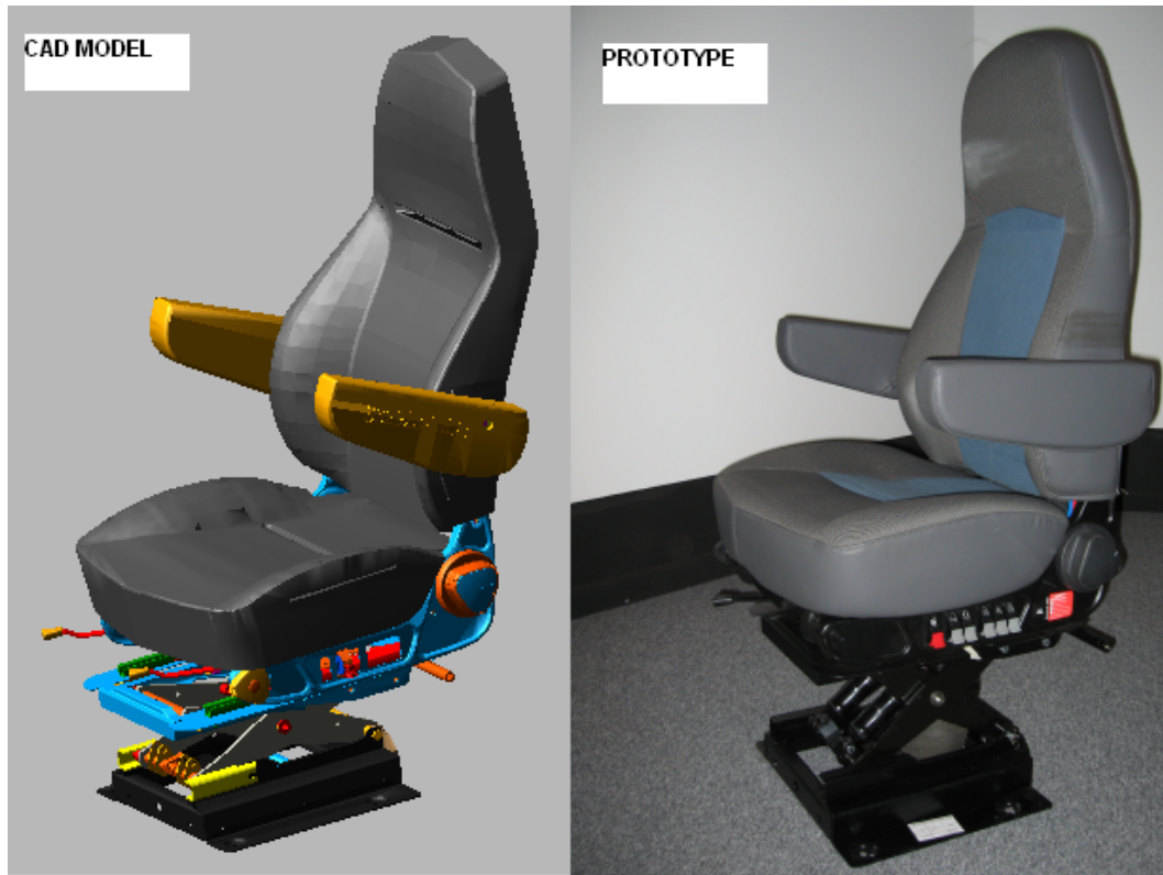
Figure 5.1: CAD model imported into ADAMS and Prototype photo
