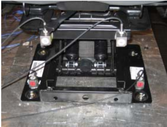
Figure 4.5a: Seat test stepup:Accelerometer instrumentation front view
