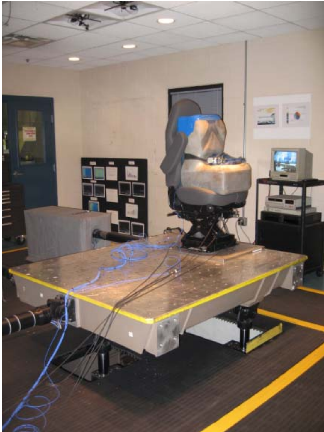
Figure 4.6: Complete seat test setup
