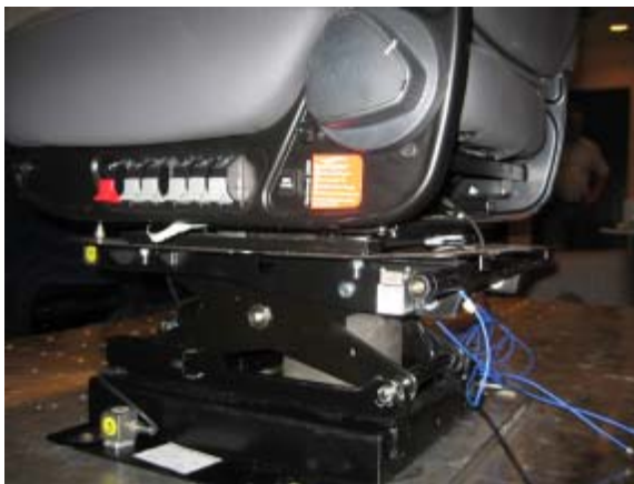
Figure 4.5b: Seat test stepup:Accelerometer instrumentation left view
