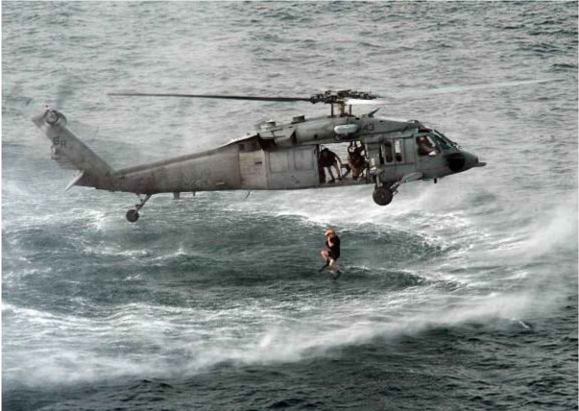
Figure A-26: MH-60S search and rescue swimmer deployment from a 15 foot hover
