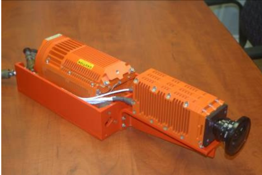
Figure A-10: Multi-System Controller with Long-Term Test Capability Camera
