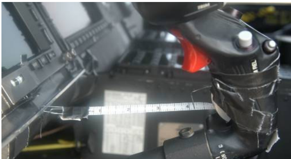
Figure A-15: Longitudinal cyclic displacement measurement installation
