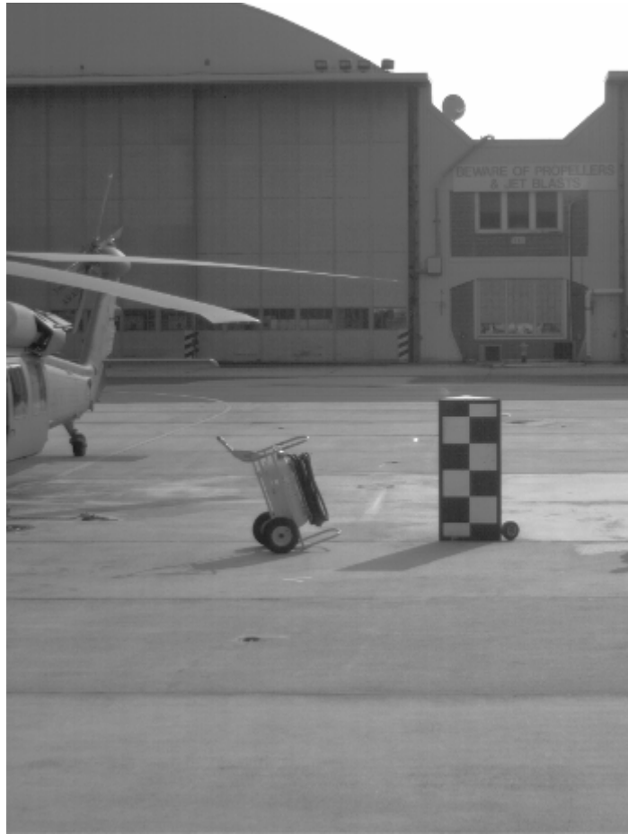
Figure A-13: Vertical calibration pole in position @ 1 blade radius from the rotor hub, rotors static
