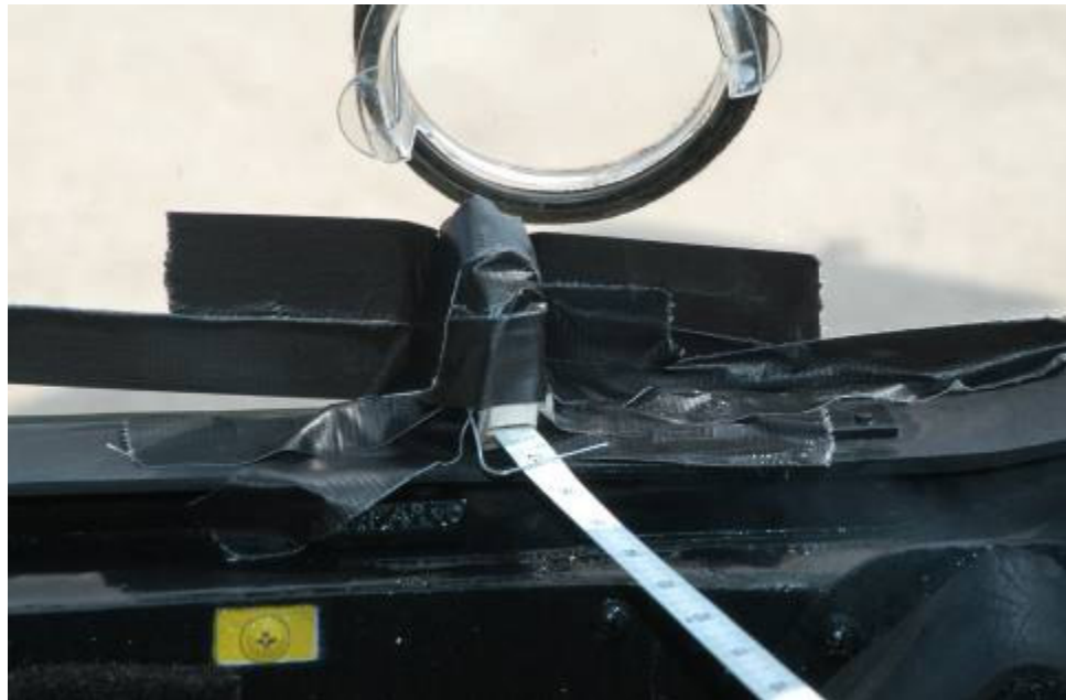
Figure A-17: Lateral cyclic displacement door-mounted measuring tape installation
