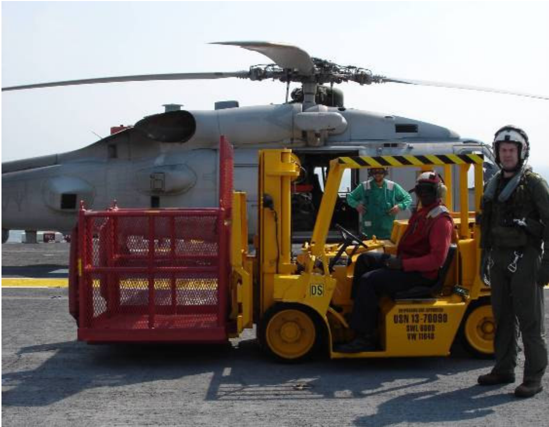
Figure A-28: Lifting LK6SLP low profile forklift under a static H-60 rotor blade at the 3 o'clock position, next to a 6 foot 1 inch person
