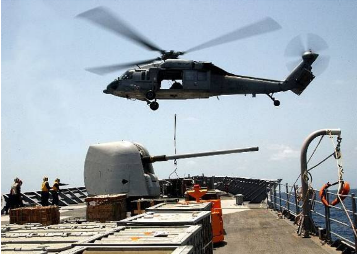
Figure A-25: Vertical Replenishment with the MH-60S
