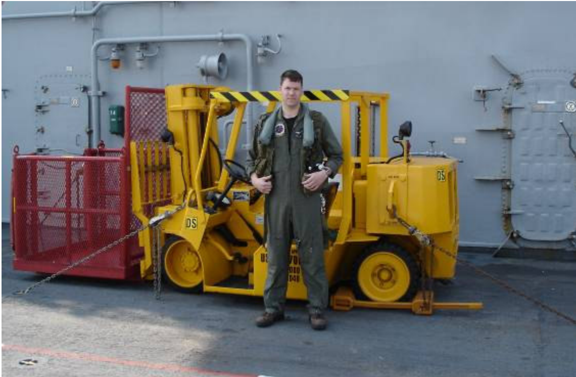
Figure A-27: Liftking LK6SLP low profile forklift next to a 6 foot 1 inch person
