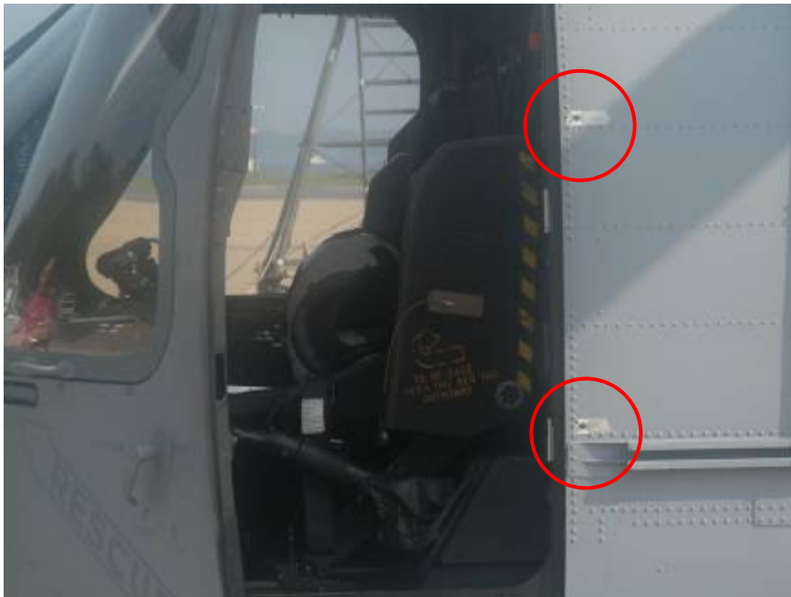
Figure A-11: Two of the surveyed aircraft reference points – copilot doorframe
