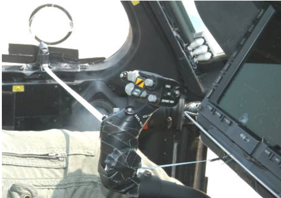
Figure A-14: Copilot cyclic control stick, cloth measuring tape configuration
