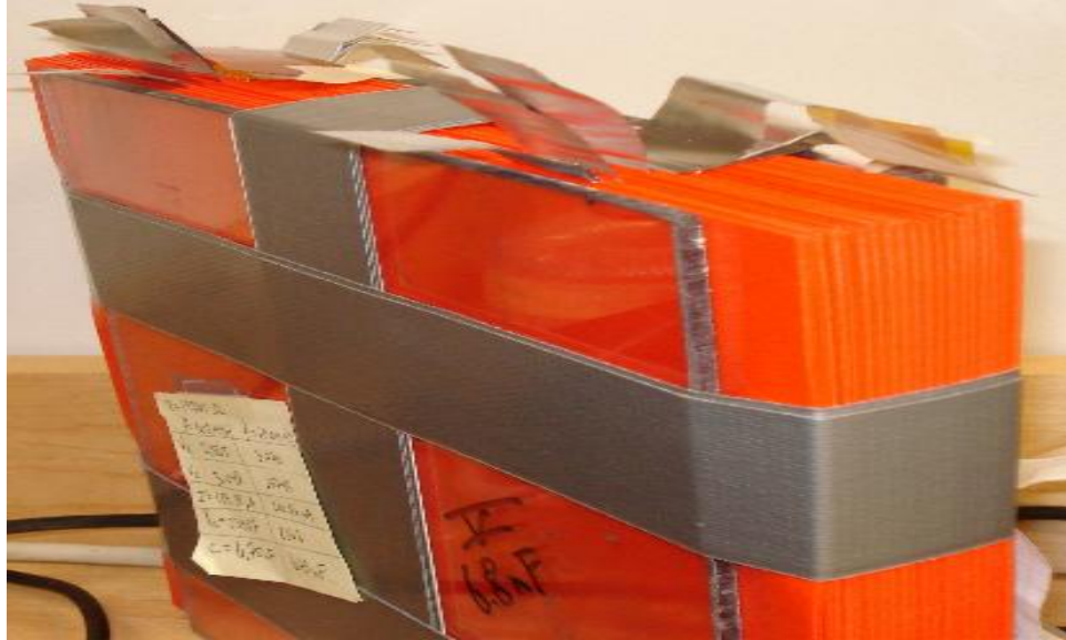
Figure 4.21. Alternate high voltage variable capacitor.
