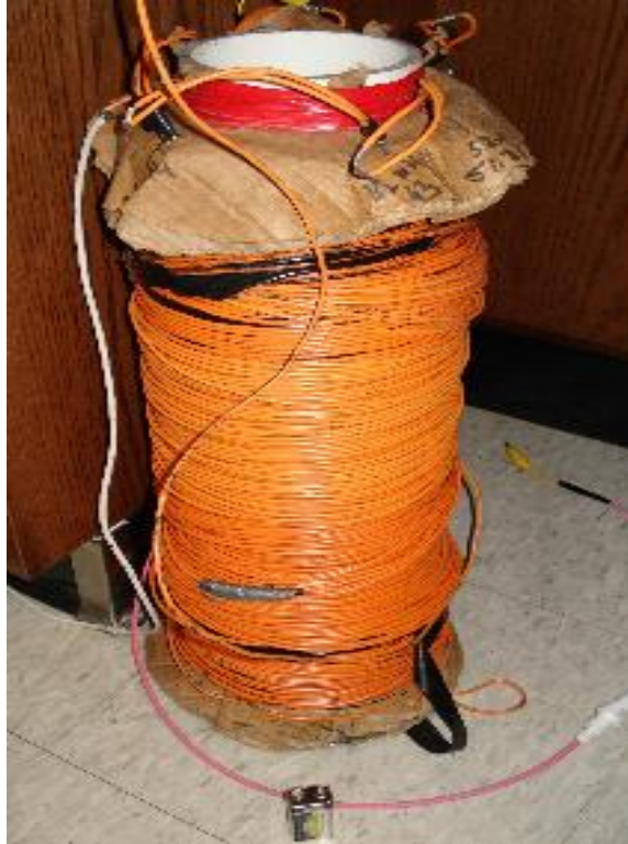
Figure 4.13. Impedance matching inductor, built by Chen [27].
