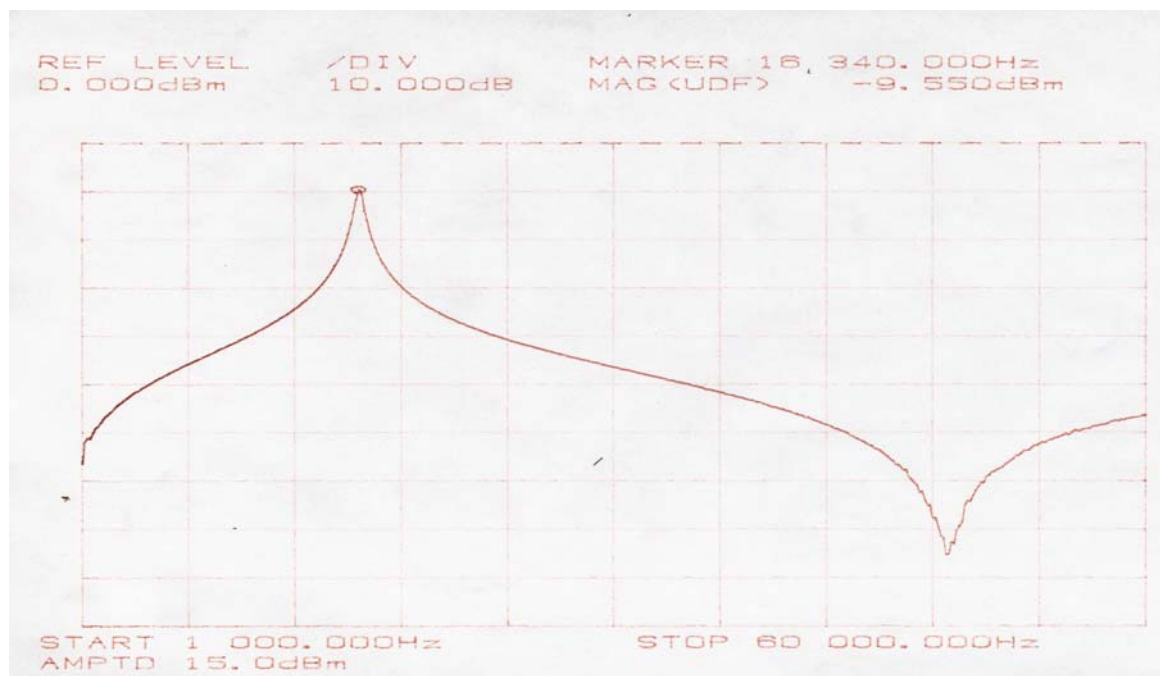
Figure 4.1. Flyback transformer frequency signature.
