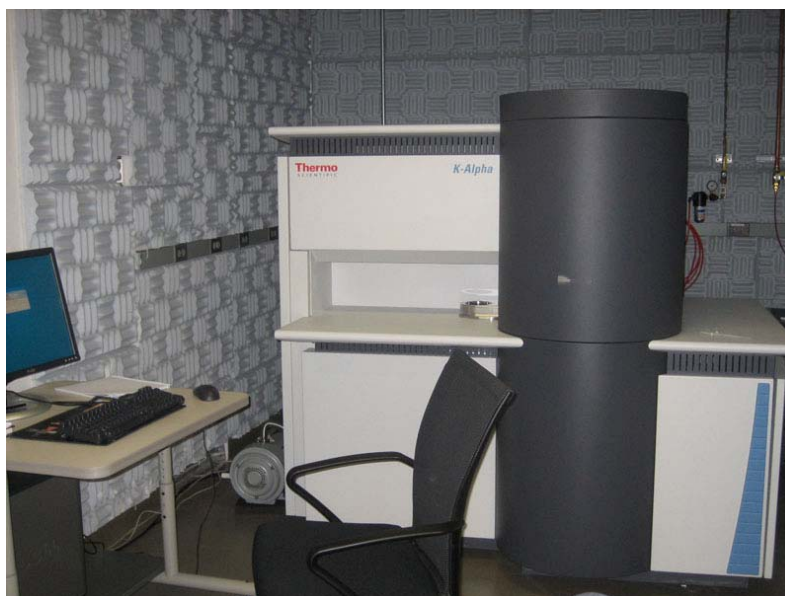
Figure 2.5. Thermo K-Alpha XPS located at Oak Ridge National Laboratory.
