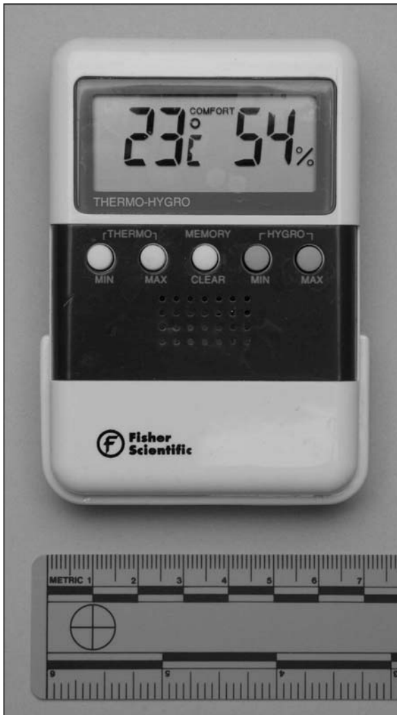
Appendix 1-5: Temperature-Hygrometer (Fisher Scientific, Suwanee, Georgia, USA) “15cm (6in) ruler included for scale”:
