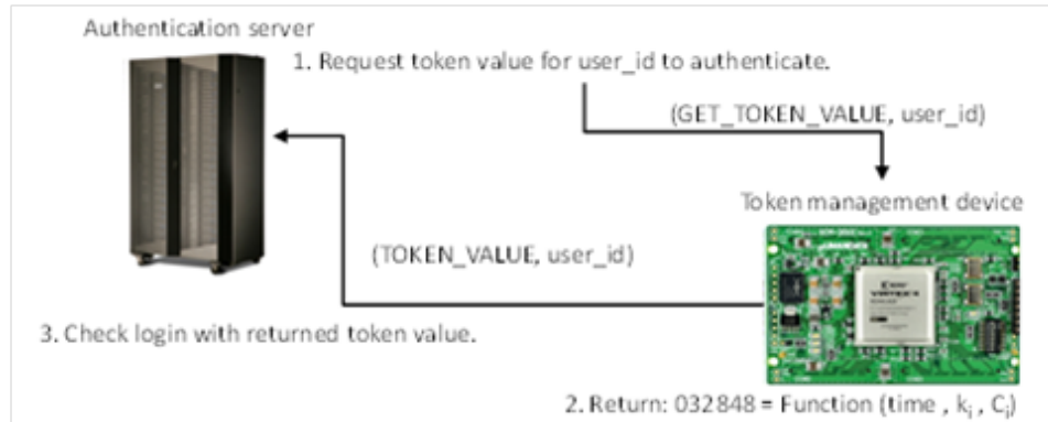
Figure 7.2: Secure Identity Management through Hardware-enforced Security Policies.
