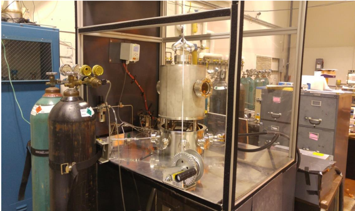
Figure 28: System with the bell jar lifted off of the base well via the winch and pulley.
