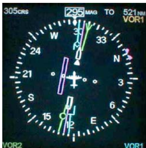
Figure 3.3. CP140 EHSI in the VOR navigation mode.
