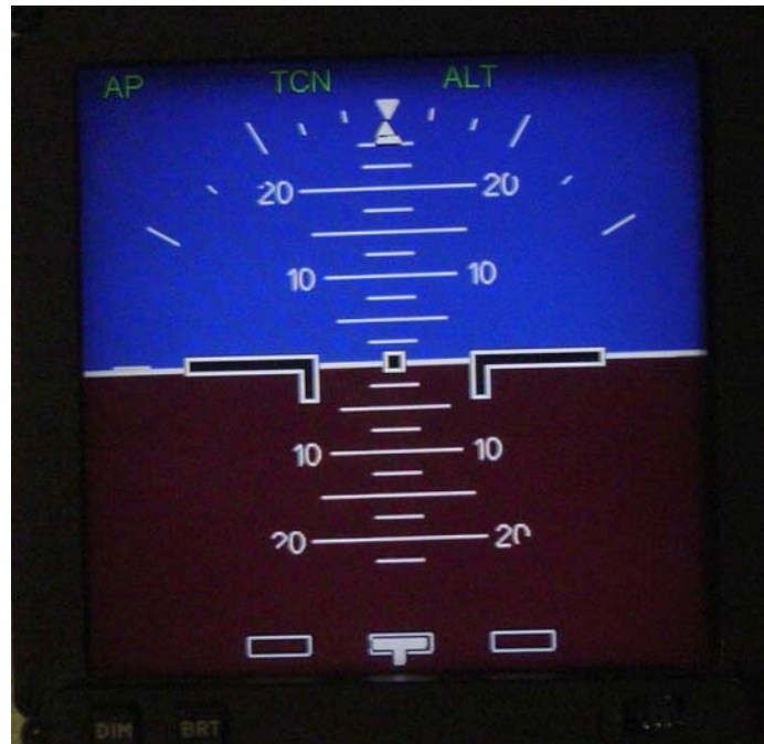
Figure 5.11. CP140 EFDI showing the AP engaged and coupled.
