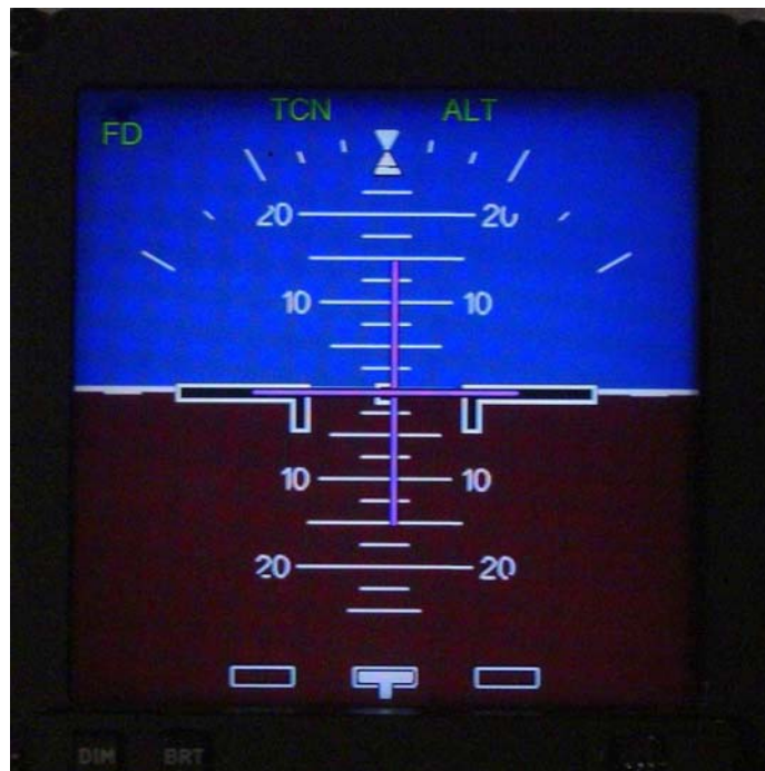
Figure 5.12. CP140 EFDI showing FD only.
