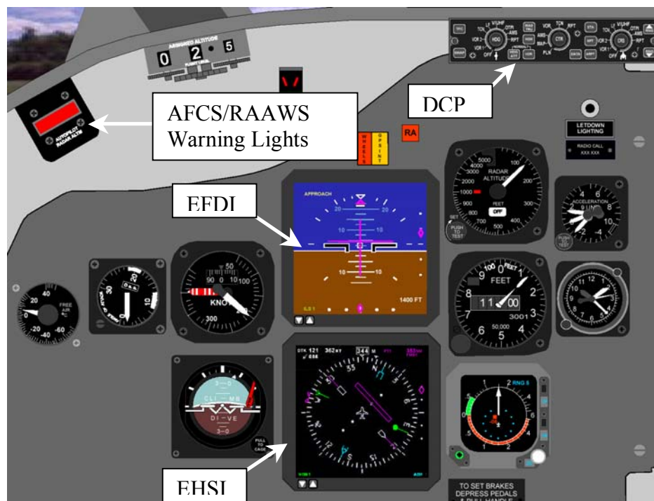
Figure 5.6. Pilot's instrument panel equipment layout showing the AFCS/RAAWS warning lights in the top left hand corner.
