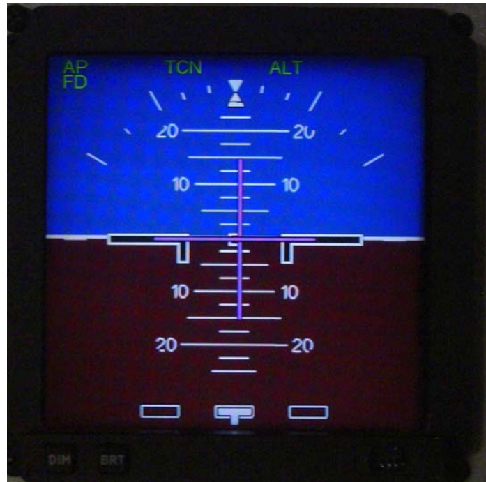
Figure 5.13. CP140 EFDI showing both the AP and FD in an uncoupled state.
