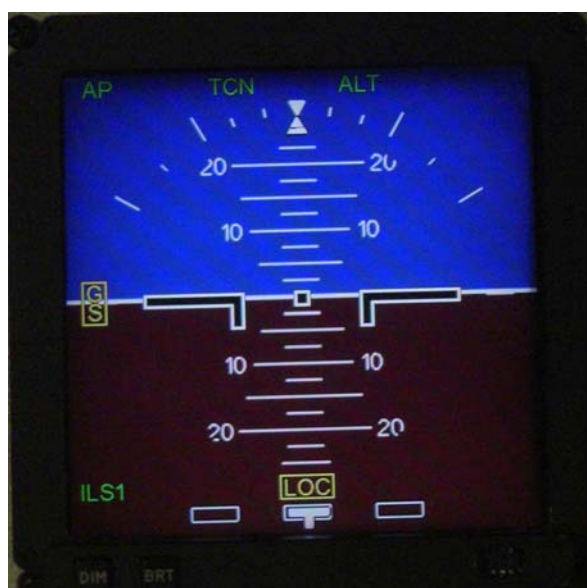
Figure 5.9. CP140 EFDI showing both TACAN and ILS approach symbology.
