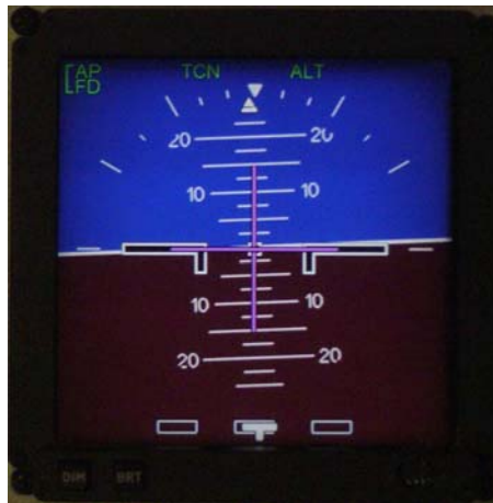
Figure 3.2. CP140 EFDI showing AFDS status combination 5 from Table 3.1.
