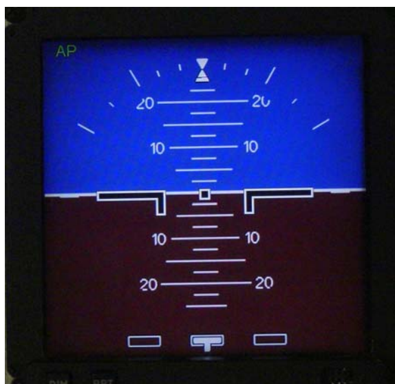
Figure 5.10. CP140 EFDI engaged in the basic AP mode.
