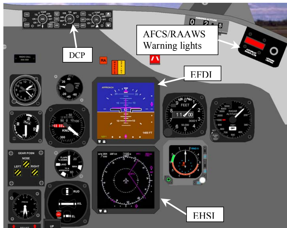
Figure 5.7. Co-pilot's instrument panel equipment layout showing the AFCS/RAAWS warning lights in the top right corner.
