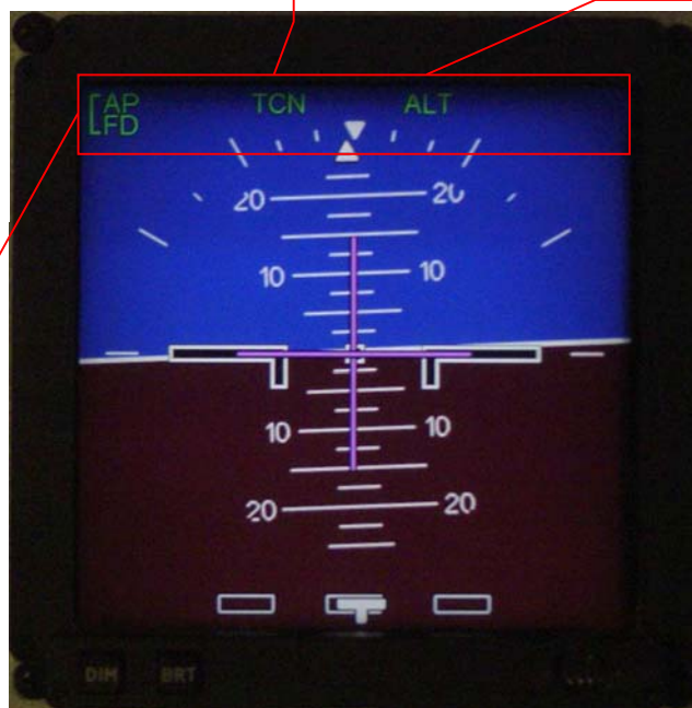
Figure 5.1. CP140 EFDI showing the AP and FD System status.
