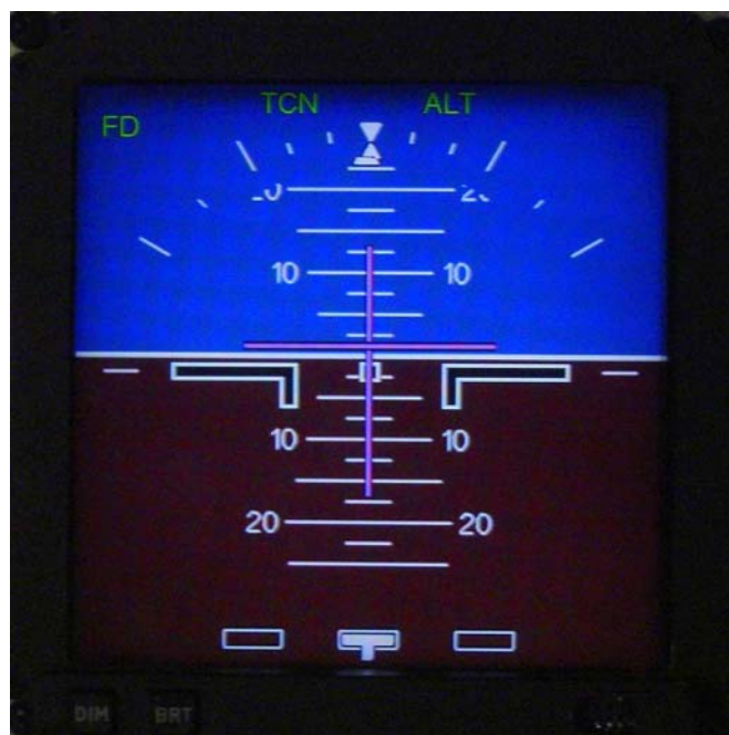
Figure 5.5. CP140 EFDI showing AFDS status following AP disengagement.
