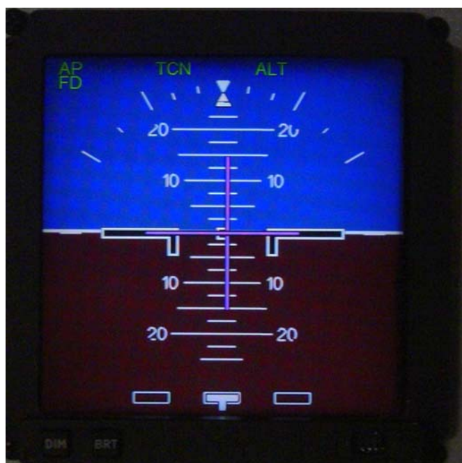
Figure 5.4. CP140 EFDI showing AFDS status prior to AP disengagement.
