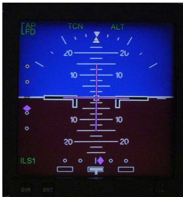
Figure 5.8. CP140 EFDI with approach course selected to TCN on the DCP.
