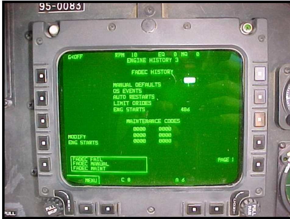
Figure 4 FADEC Messages of MFD
