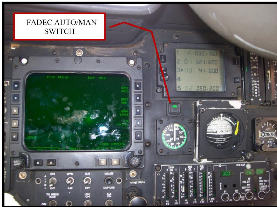
Figure 3 FADEC Switch in AUTO Mode
