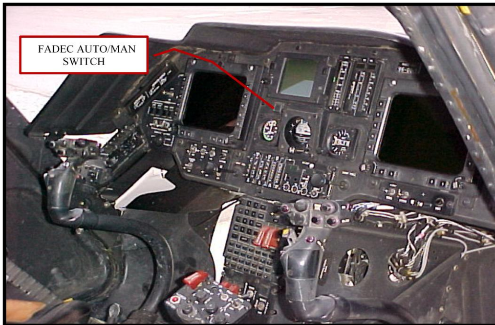
Figure 2 FADEC AUTO/MAN Switch
