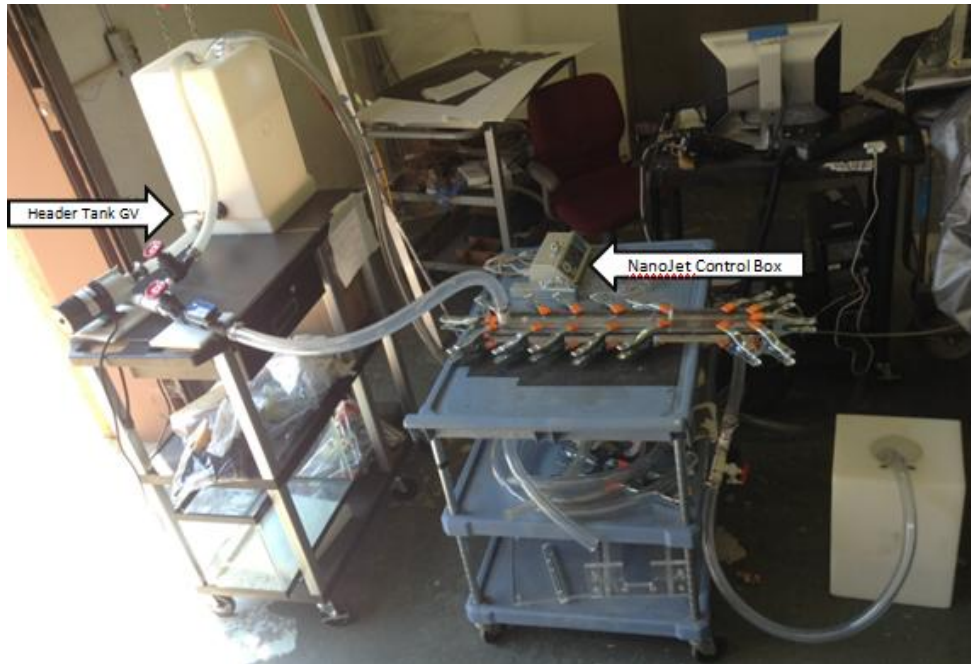
Figure 33: Header Tank and Control Box Identification
