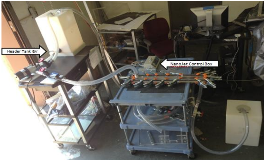
Figure 21: Test Section and Flow Loop Setup.
