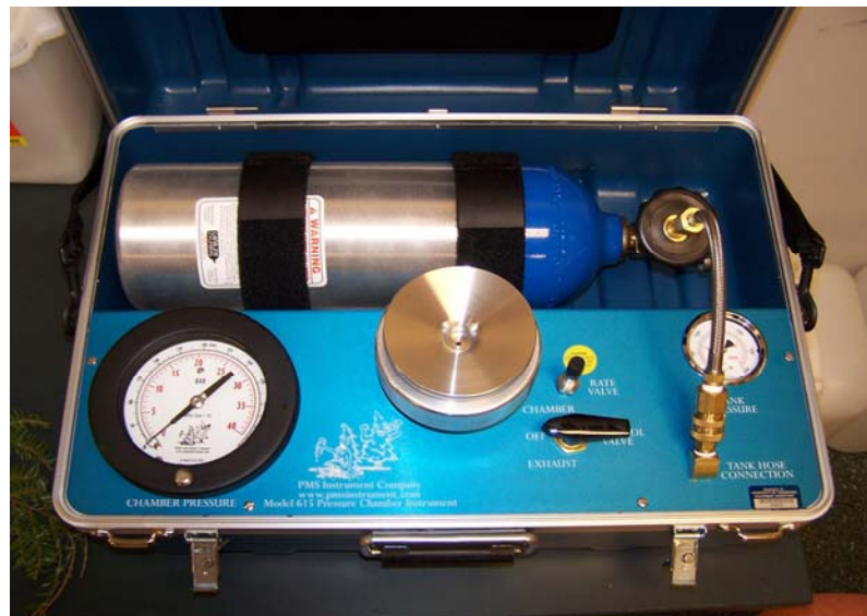
Figure 6. PMS pressure chamber used to extract sap from eastern hemlock samples to test for imidacloprid concentrations.
