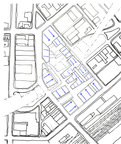
figure 39: Rainwater catchment Runoff from the roofs of the school is collected and stored in cisterns. The water is later used to meet graywater and landscaping needs.
