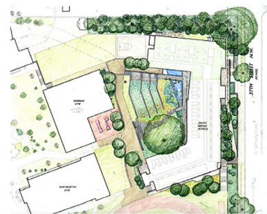
figure 35: Sidwell Friends School plan Sidwell Friends School uses many sustainable strategies including the constructed wetland/ biofilter/ rain catchment system located in the courtyard.
