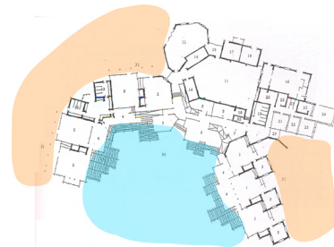
figure 62: Woodlea Primary School, outdoor spaces outdoor spaces are grouped by use: loud (orange) and quiet (blue)
