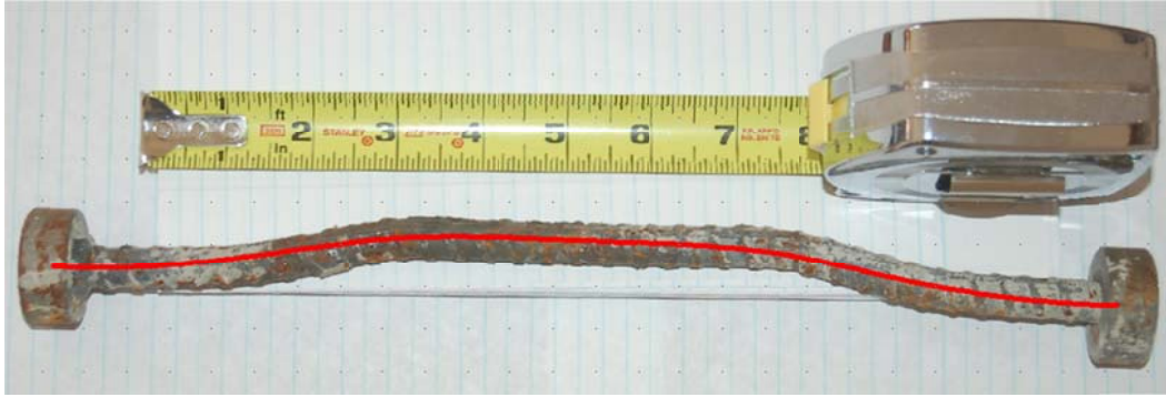
Figure 27: ST-0 lacer bar from loaded side compared to the adjusted model
