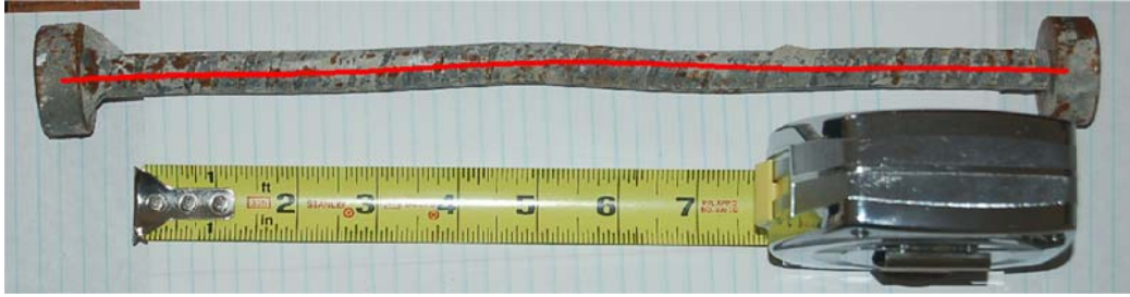
Figure 31: ST-0 lacer bar compared to the adjusted model deflection
