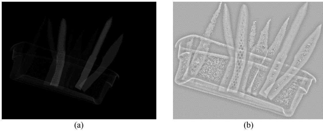
Figure 3.4 Standard measure technique. (a) Original scan and (b) its standard measure enhanced version.
