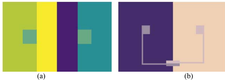
Figure 5.2 Simultaneous contrast can make (a) the same colors look different, or (b) different colors look the same [Taylor and Murch, 1986].
