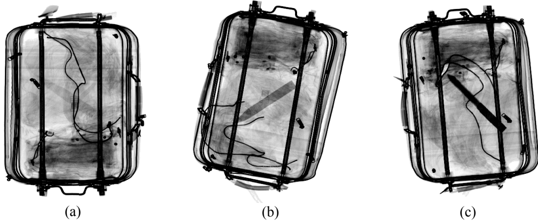
Figure 5.7 Enhanced version of Figure 5.4 produced by using original + negative + h-dome + contrast stretching.
