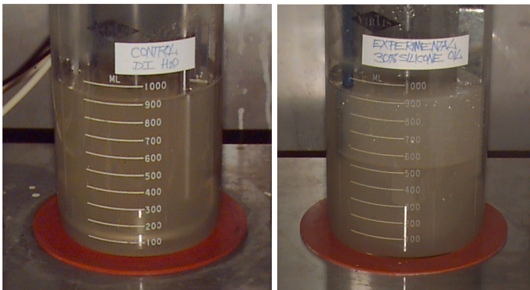
Figure 3.3. Control reactor versus 30% silicone oil reactor during operation. The agitation was turned off before this photo was taken.
