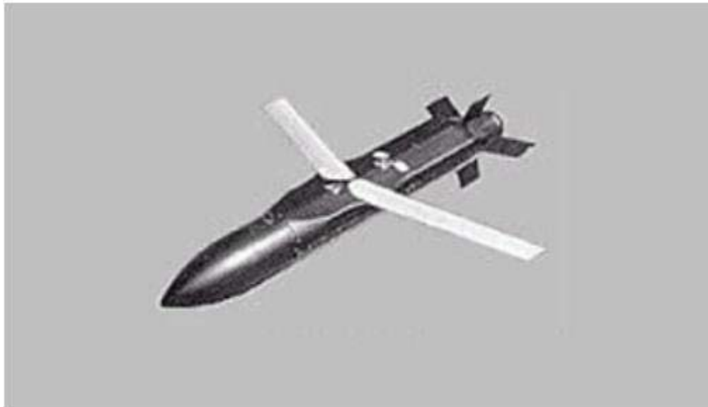
Figure 1-3: Sampson Air Launched Decoy
