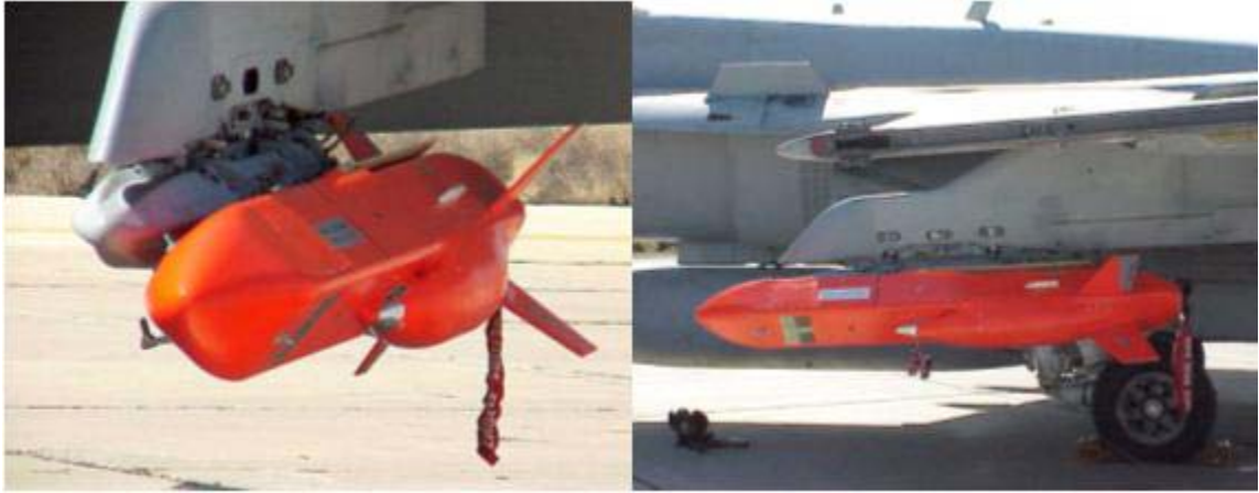
Figure 3-10: ITALD Mounted on ITER Shoulder Station
