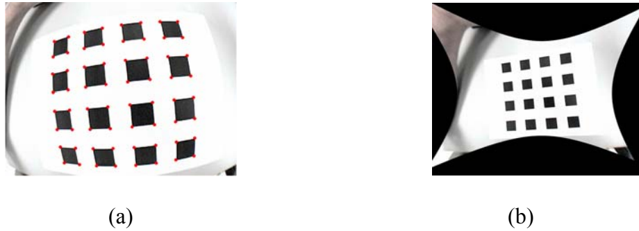
Figure 4.3: An example of a planar calibration model. (a) Original calibration target with the control points shown in red and (b) corresponding image corrected towards a perspective projection.
