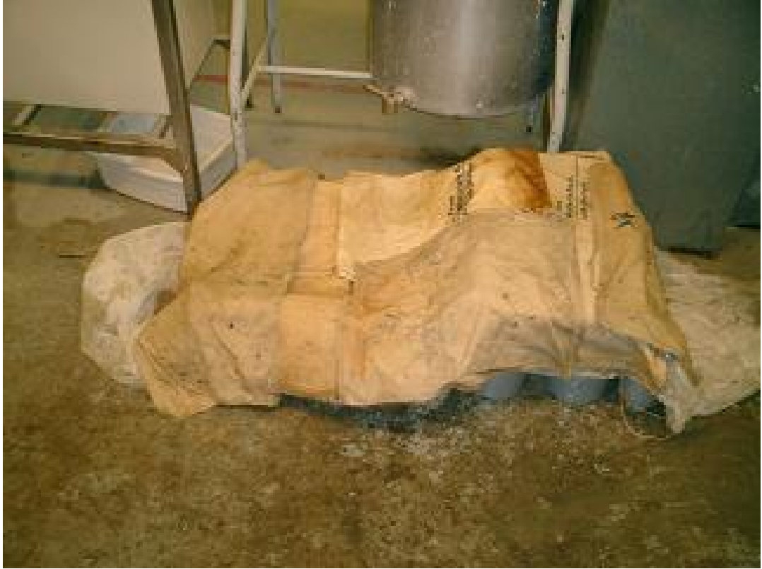
Figure 3.2 Specimens Topped with Wet Burlap Sacks.
