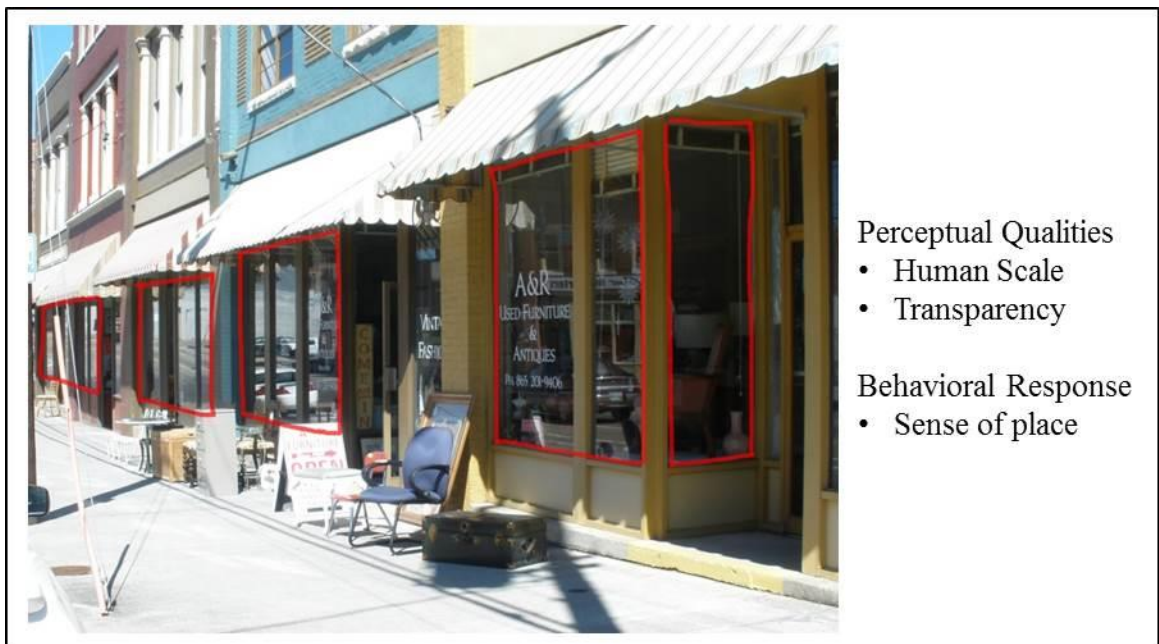
Figure D.28: (b) – Human Scale and Transparency / Sense of place and Sense of safety Objects for sale along street promote interest and provide character. Windows at street level allow for opportunities to observe people creating further interest.
