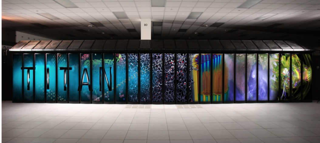
Figure 1.1: The Oak Ridge Leadership Computing Facility (OLCF) is home to Titan, the world’s most powerful supercomputer for open science with a theoretical peak performance exceeding 20 petaflops. Image courtesy Oak Ridge National Laboratory.
