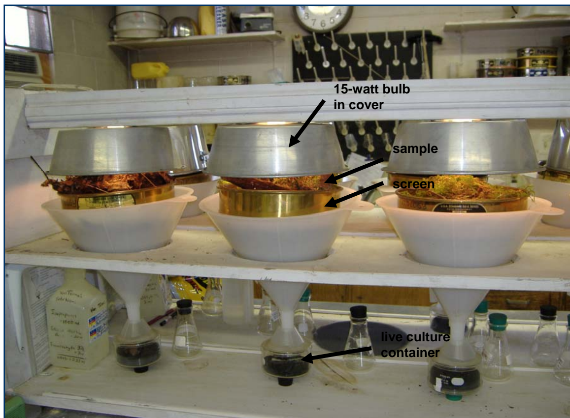
Figure 3. Tullgren funnels used to extract live specimens.
