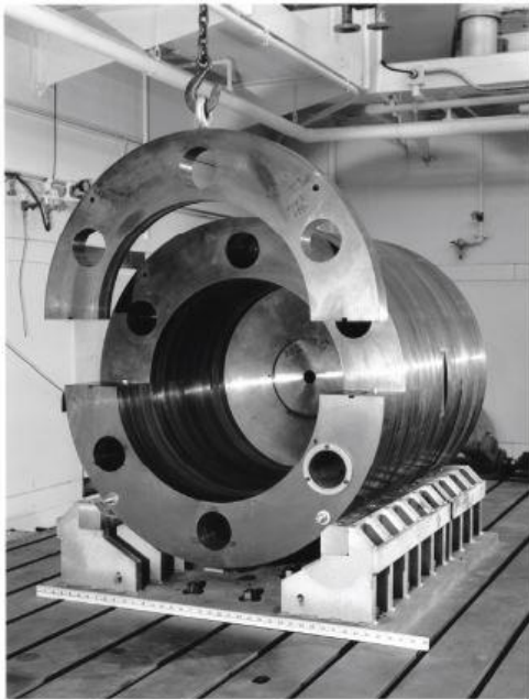
Figure 14. Assembly of the Big Ten Reflector Segments for IMF-007 [6]
