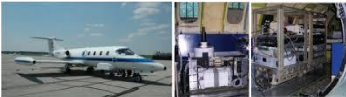
Figure 1.1 (Left) NASA Glenn-Lear 25 aircraft. (Middle) Lidar installed on the aircraft with sensor head assembly and (Right) dual aircraft racks [8].
