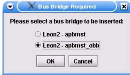
Figure 4.5-3: AHB-APB Bus Bridge Dialog Box
